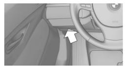
The OBD socket for checking components definitive in terms of the composition of the exhaust emissions is on the driver's side.
