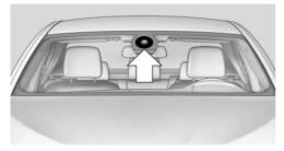
The camera is in the area of the base of the rear-view mirror.
