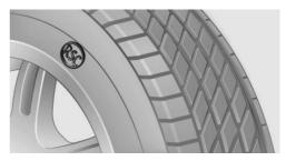
RSC marking on the tyre side wall.
