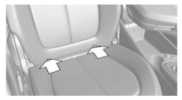
The brackets for the lower ISOFIX anchors are located in the gap between the seat and back-rest.
