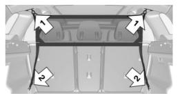
3. Hang the luggage net with the two lower hooks into the respective upper lashing eyes in the boot, arrows 2.
