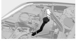
Turn the bulb holder anticlockwise and remove.
