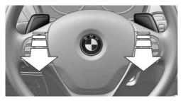
Shift paddles on steering wheel enable fast gearshifting without taking hands off steering wheel.
