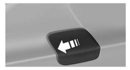
2. Turn the fuel tank cap anticlockwise.
