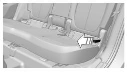
Pull loop and remove pressure on backrest as required.
