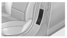
The tyre inflation pressures for the tyre sizes categorised by the vehicle manufacturer as suitable for the respective vehicle type can be found on the door pillar of the driver's door.
