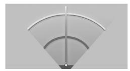
The distance between the trailer and the trailer tow hitch can be estimated with the aid of two static circular segments.
