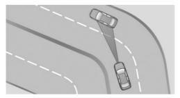
When your vehicle is approaching a bend, the angle of the bend may cause the system to respond temporarily to vehicles in the other lane. A possible reduction in the vehicle's speed by the system can be compensated for by briefly accelerating. When the accelerator pedal is released again, the system will resume control of the vehicle's speed.
