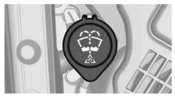
All washer jets are supplied from one tank in the engine compartment.
