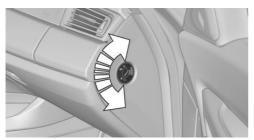
The front and side airbags for the front passenger can be deactivated and reactivated using the integrated key from the remote control.
