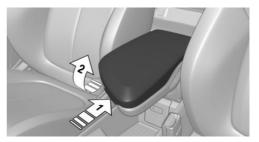
Press the button, arrow 1, and fold the centre armrest upwards, arrow 2.
