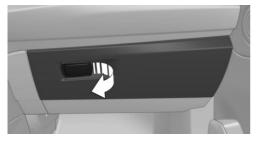
Pull the handle. The lighting in the glove box comes on.
