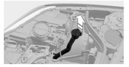
2. Turn the cover anticlockwise and remove.
