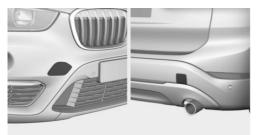
Press the marking on the edge of the cover to press it out.
