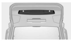
The recessed handles in the tailgate lining make it easier to pull the tailgate down.
