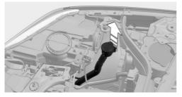
Turn the bulb holder anticlockwise and remove.
