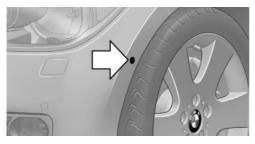
Ultrasonic sensors to measure parking spaces are located on side of vehicle.
