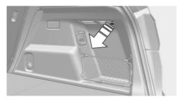
Pull the green tag with the fuel pump symbol. Fuel filler flap is unlocked. Briefly press rear edge of fuel filler flap to open, see page 196.
