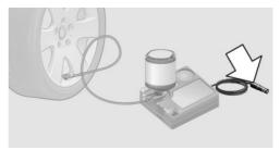
7. Switch on the compressor with the ignition switched on or the engine running.
