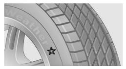
Certain makes of tyre are recommended by the manufacturer of your vehicle depending on tyre size. These can be seen by the asterisk on the side wall of the tyre.
