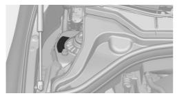
The vehicle identification number is in the engine compartment.
