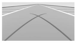
The turning circle lines can only be shown in the image from the rear-view camera together with driving lane lines. The turning circle lines show the course of the smallest possible turning circle on a level road surface.
