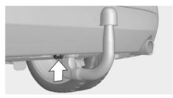
There is an eye on the trailer tow hitch bracket for attaching the trailer securing cable.
