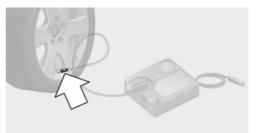
3. Plug the connecting hose directly into the compressor.
