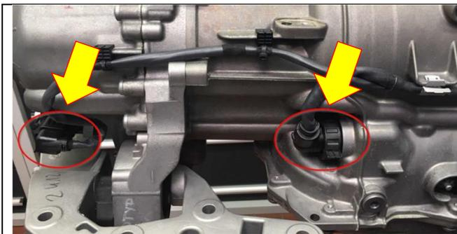
6. Disconnect the transfer case and transmission 12 V connectors.
