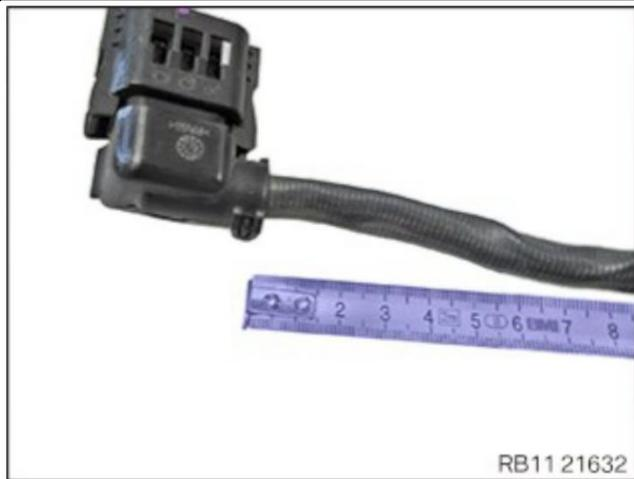
12. Position the tape measure on the connector housing.
