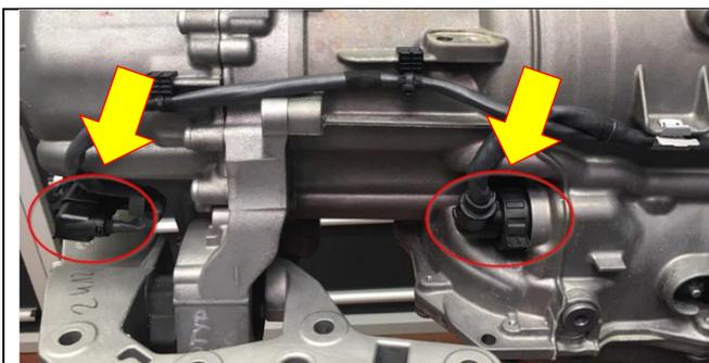
6. Disconnect the 12 V connectors from the transfer case and transmission.
