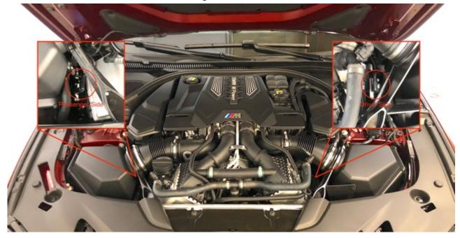
Step 2: Install the Harness by unclipping the original harness and reconnect it to the RaceChip harness. Unclip the harness by using the flat screwdriver to undo the white locking tab first, then press and pull. Then insert the male plug from RaceChip Harness to the sensor and origina male plug to RaceChip Harness female plug.
