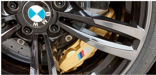
The rotating masses in M Carbon ceramic brakes are approx. 30 lbs lighter compared with standard M Compound brakes. On the other hand, these brakes are dimensioned to offer significantly more in terms of performance. So on the racetrack in particular, the M Carbon ceramic brake is first choice.
