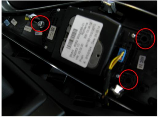
8. Pop the shifter boot out by prying from the front then sliding out the back. Then pull it up so it is out of the way. Remove the rest of the center console by prying up the trim ring shown below. Start from the arm rest and pry it up evenly before pulling it out.
