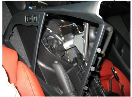
10. Now remove the cup holders by 2 screws torx #20 (circled). pull up from the back and slide back towards the arm rest. Then let is hang over the side.
