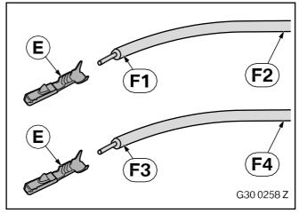
Cut the GREY **F** cable so that there is a 7m length to the **F1/F2** and a 5m length to drain the **F3/F4.**
