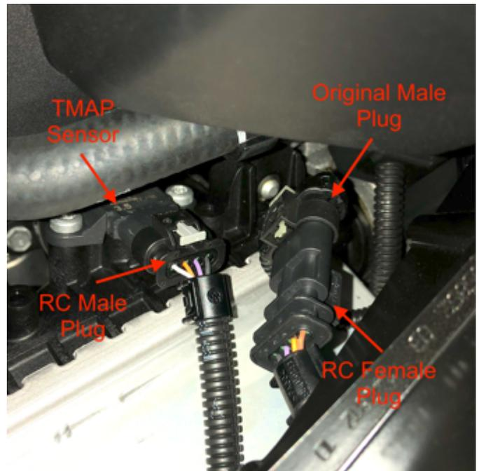
Step 3: Route the harness and mount the RaceChip Unit using supplied mounting clips and zip ties. Cut the excess of zip ties using wire cutter or scissor.
