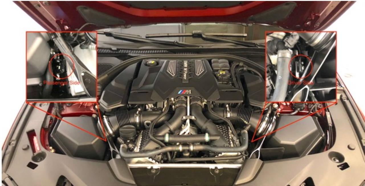
Step 2: Install the Harness by unclipping the original harness and reconnect it to the RaceChip harness. Unclip the harness by using the flat screwdriver to undo the white locking tab first, then press and pull. Then insert the male plug from RaceChip Harness to the sensor and original male plug to RaceChip Harness female plug.
